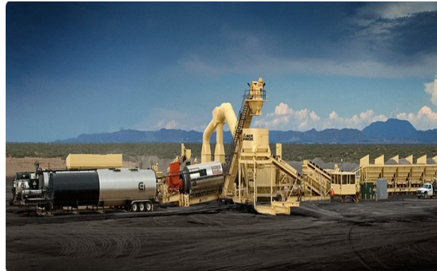
Drum Mix Plant
