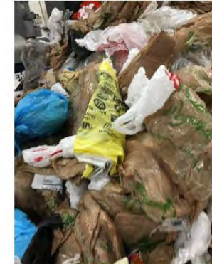
Test Run 2: Front Store Material (customer drop off) Some Paper, Pouches, Mixed Material Contamination Colored bags
