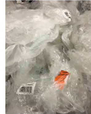
Test Run 1: Back Store Material Significant Paper Label Contamination Some colored bags
