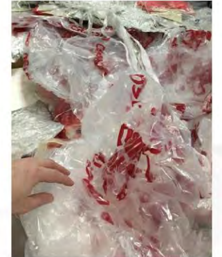
Test Run 3: Back Store Material Limited Paper Label Contamination Red printed large bags
