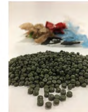
Test Run 2: Front Store Material (customer drop off) Some Paper, Pouches, Mixed Material Contamination Colored bags
