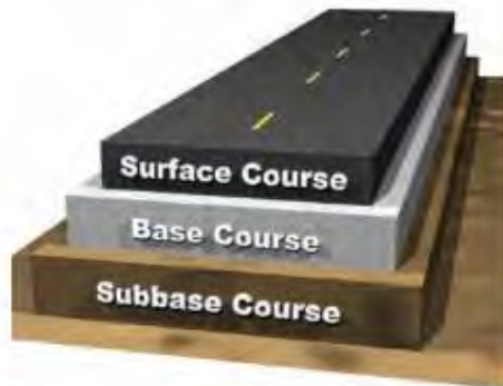
Typical Pavement Structure. Only the top of surface course would be removed and replaced as it is worn by traffic; the rest of the pavement structure remains in place.
