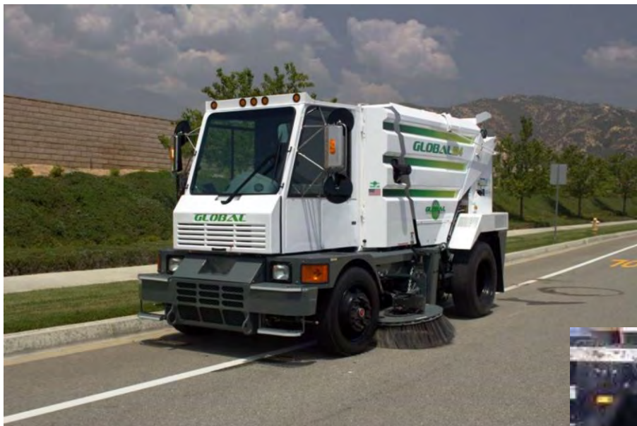
Sweeping Roads to Remove Dust
