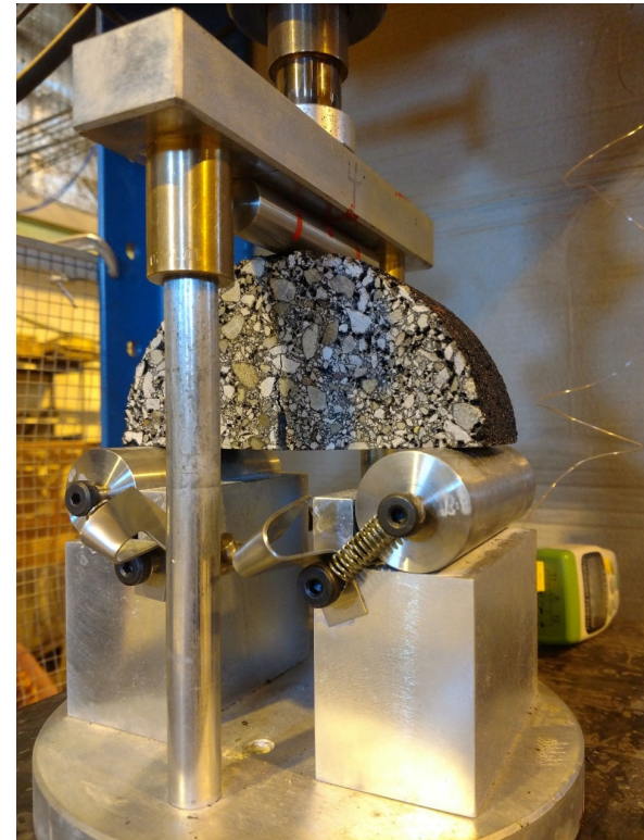
Semi-Circular Bend (SCB) Test Setup
